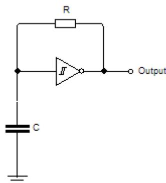
Schmitt trigger based Astable
