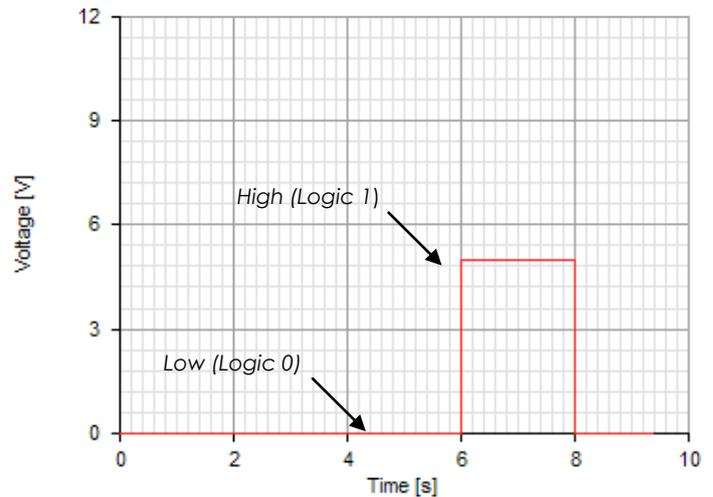
Digital signal with a high (logic 1) output voltage of 5V
