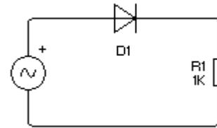
Half-wave rectifier circuit
