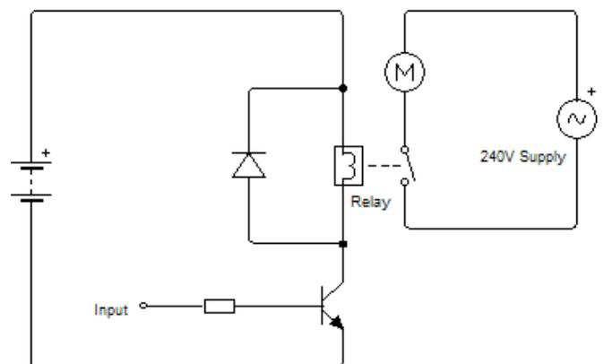
A diode being used to protect a transistor from Back EMF
