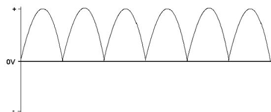
Voltage developed across the resistor
