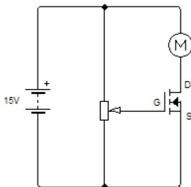
Motor speed control circuit
