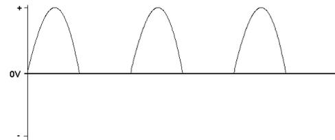
Voltage developed across the resistor
