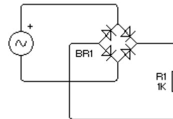
Full-wave bridge rectifier circuit
