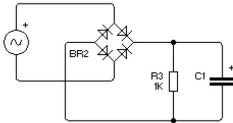
Full-wave rectifier with reservoir capacitor
