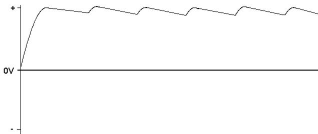
Voltage developed across the resistor (exaggerated for clarity)
