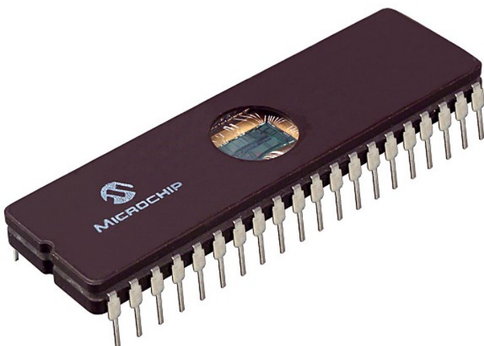
PIC Microcontroller with window showing internal integrated circuit
