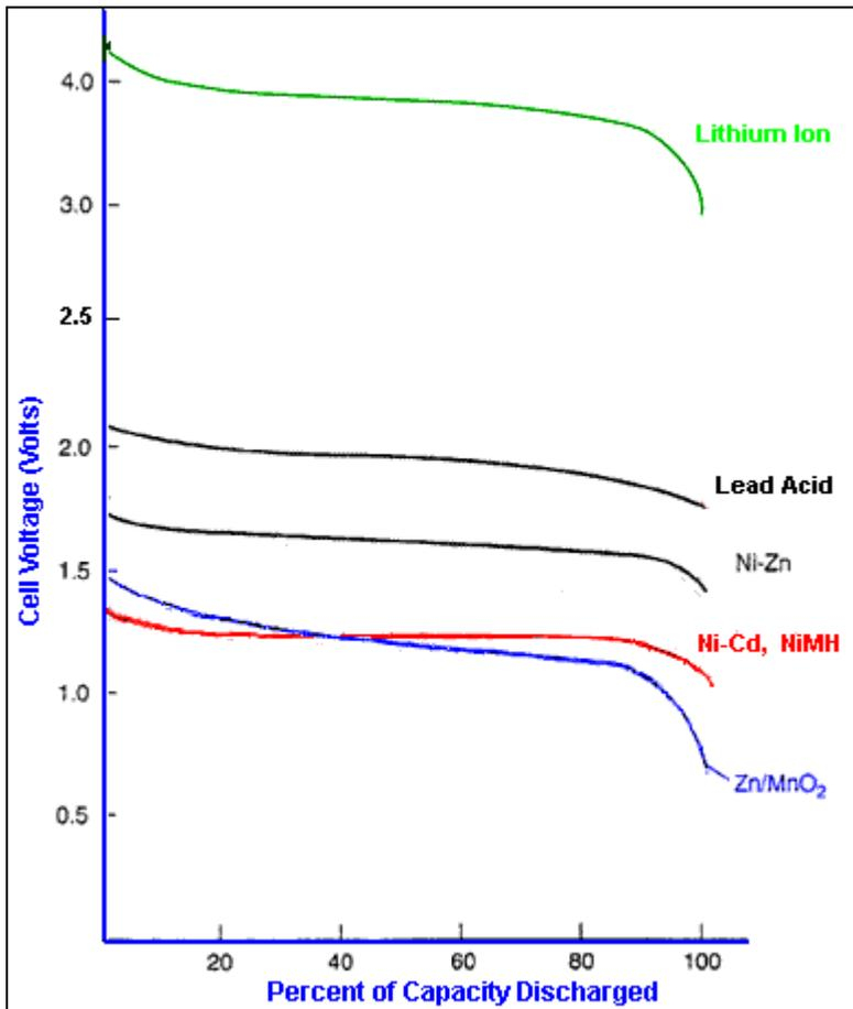
Common discharge curves of common batteries
