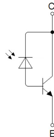
Phototransistor equivalent circuit
