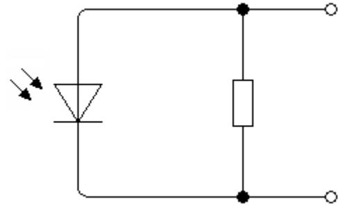
Photodiode in PV mode
