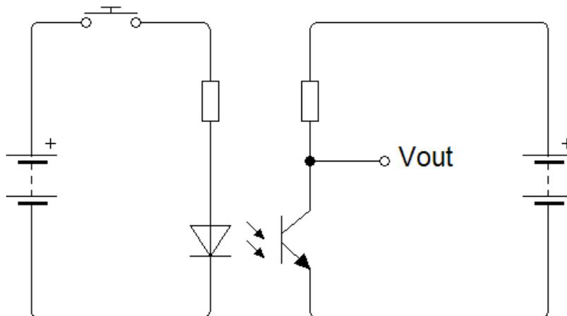
When the switch is open, no current flows through the LED and therefore it does not light up. Because of this, not light reaches the phototransistor, that will therefore be switched off and  $V_{out}$  will rise to the voltage of the battery.
